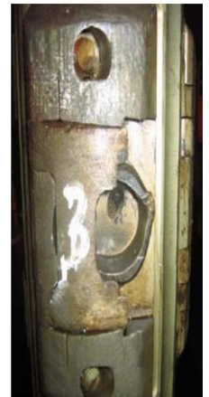
Figure 12. Limitation of RSS Type A (Push The Bit) for basement drilling
