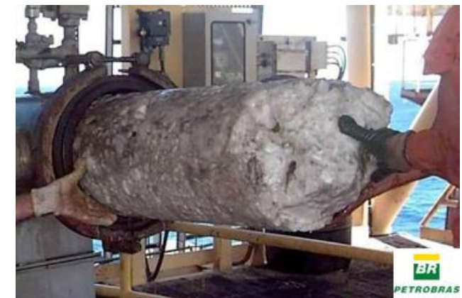
(Hydrate recovered at slug catcher-Petrobras)
