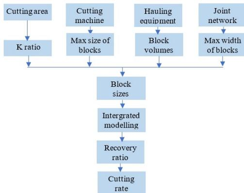
Fig 1. Flow chart to calculate suitable size for dimension stone
