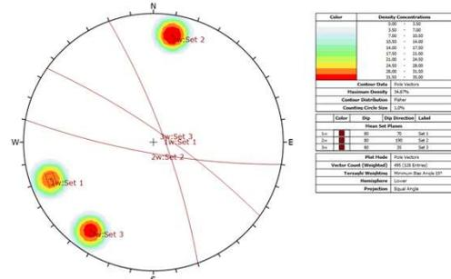
Fig. 2. Analysizing and representing joint sets for Tan Long dimension stone quarry in Binh Dinh Province
