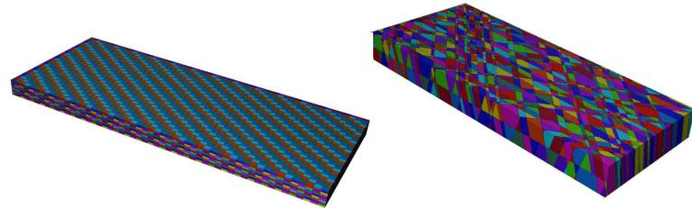
Fig. 3. Three-dimensional joint sets modelling and cutting-grid modelling for Tan Long dimension stone quarry, Binh Dinh Province.
