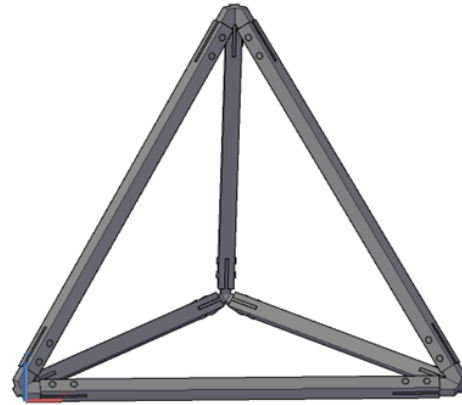
Fig. 7 Glulam Space Truss Model in AutoCAD 3D Space
