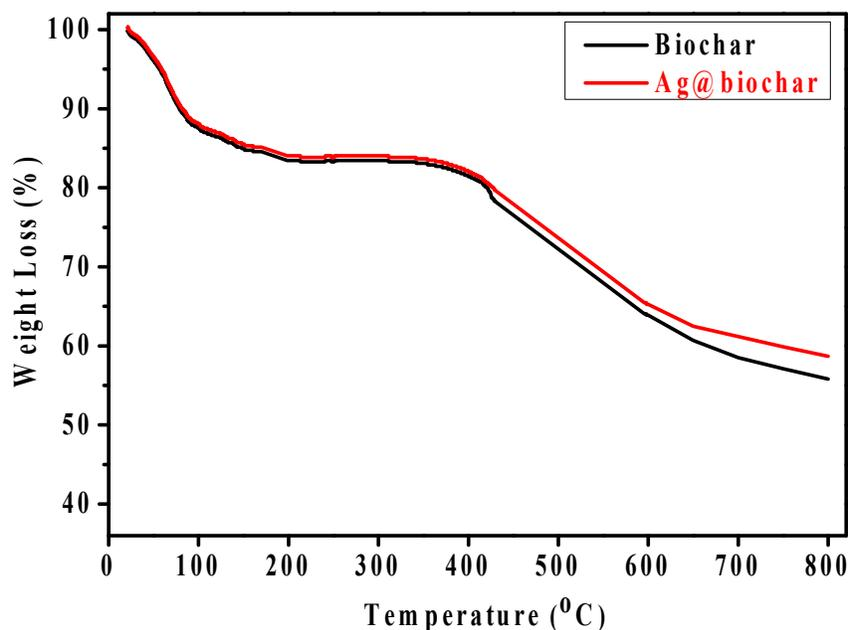
**Fig. 3.** TGA curves of biochar and Ag@biochar
