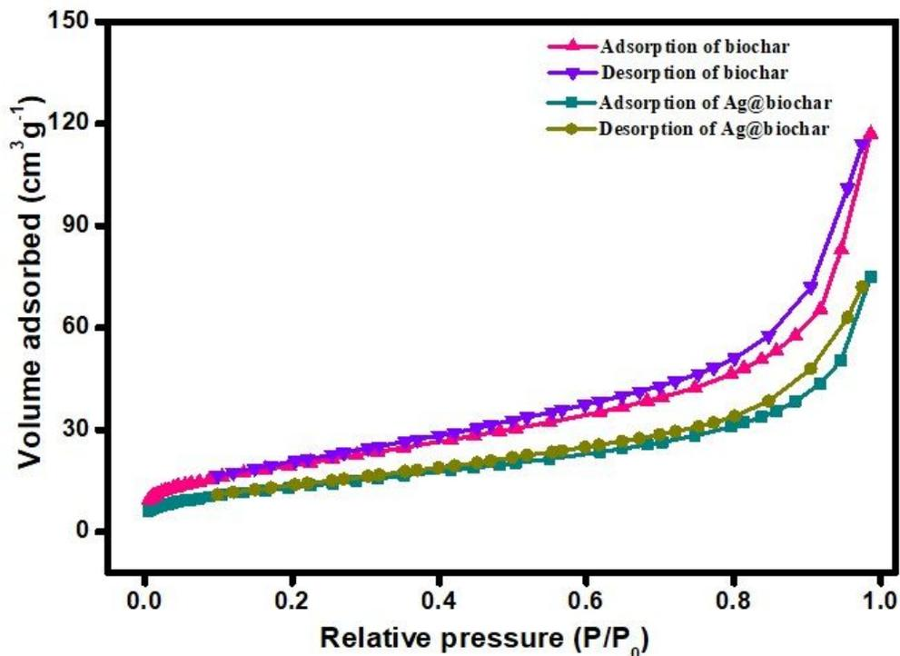
Fig. 4. N<sub>2</sub> adsorption/desorption isotherm of biochar and Ag@biochar.
