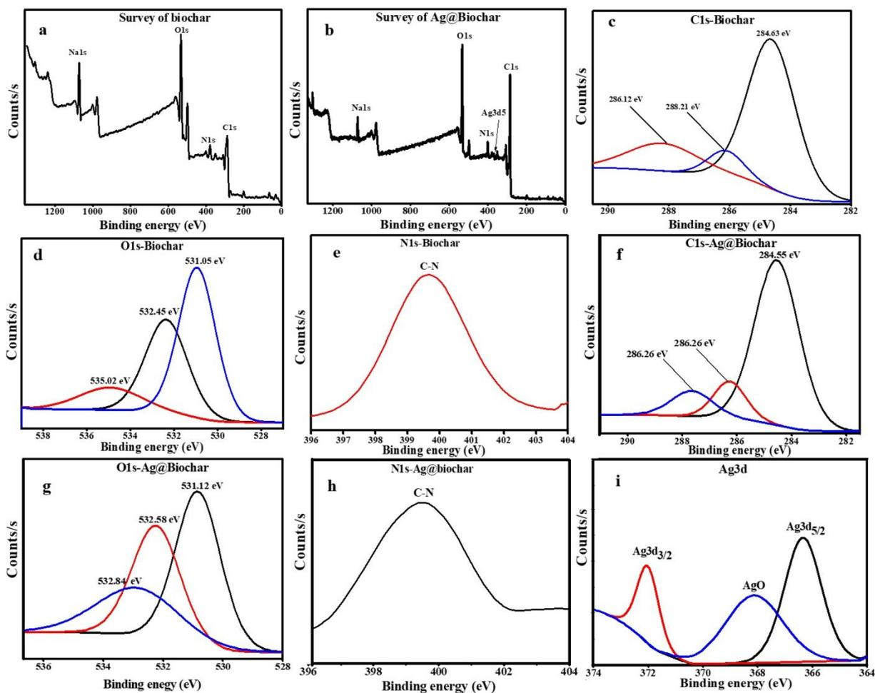
**Fig. 2.** XPS spectra for biochar survey (a), Ag-biochar survey (b) biochar C1s (c), O1s (d), N1s (e), Ag-biochar C1s (f), O1s (g) N1s (h), and Ag3d (i).
