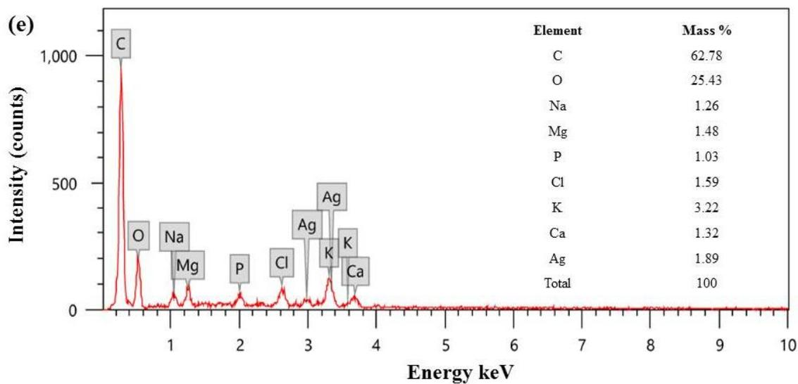
**Fig. 1.** SEM photomicrograph of (a, b) Ag@biochar, (c, d) biochar, and (e) EDX analysis.
