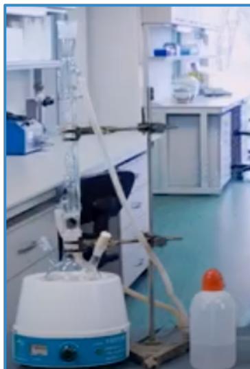
Figure 1. Reflux Distillation for preparation of polymer films
