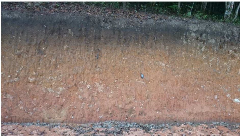
Image 3.5: Cross section of Saprock weathering crust in Ngam Lim ward
