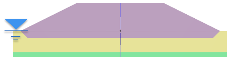
Fully fouled embankment
