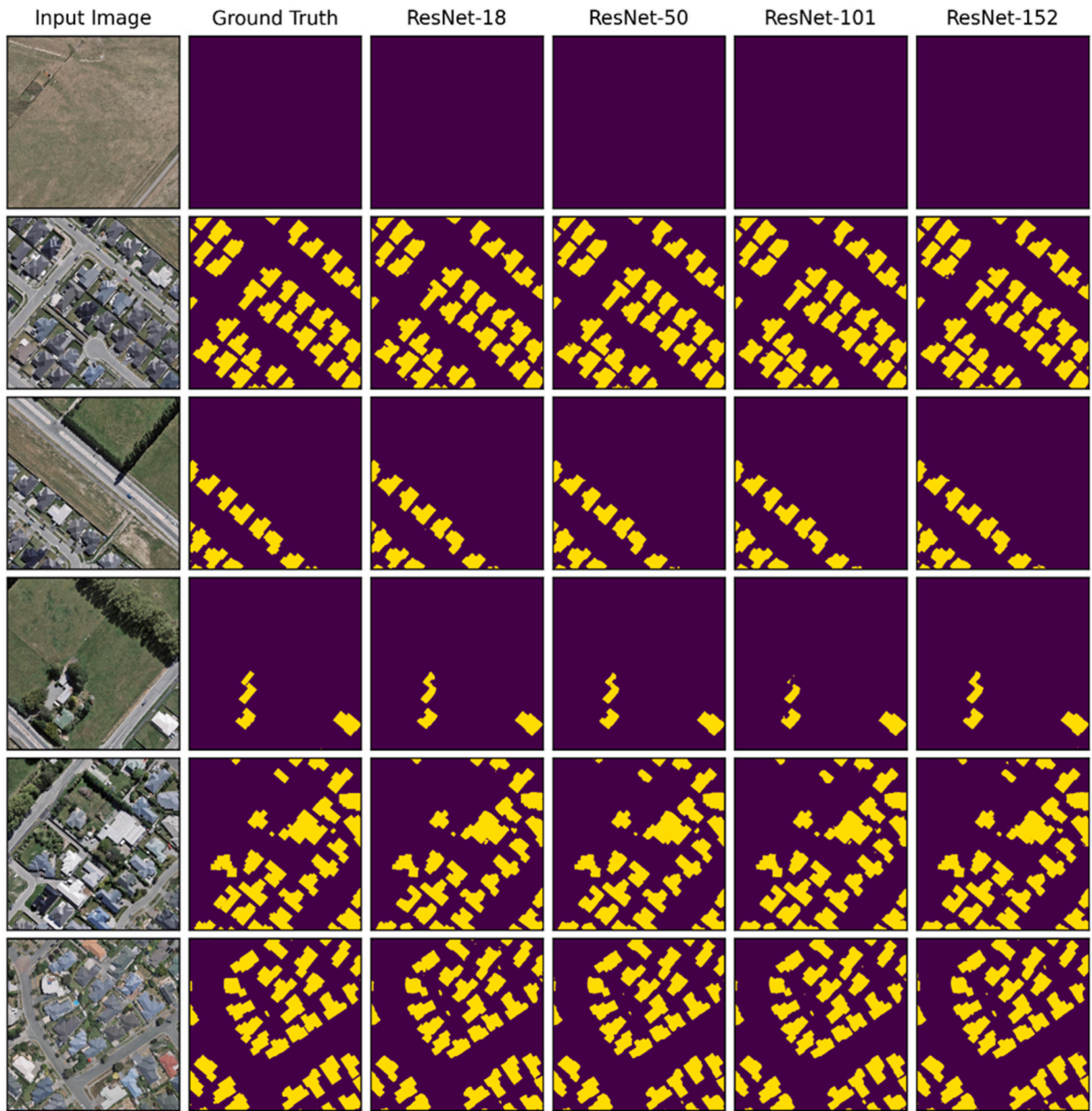
Fig. 5. Semantic segmentation results comparing different ResNet backbones (ResNet-18, ResNet-50, ResNet-101, ResNet-152) in DeepLabV3+, trained on 40 % of the WHU dataset using ImageNet pretraining and data augmentation. Each row presents the input image, ground truth, and segmentation predictions. Yellow represents buildings; purple represents background.
