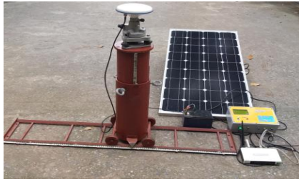
Figure 4: Real-time displacement monitoring system of works
