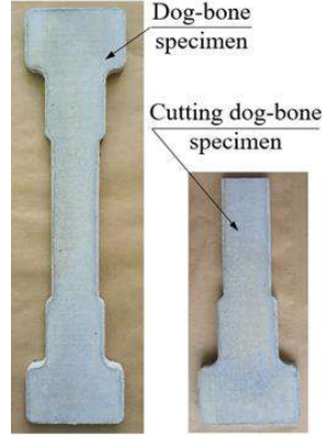
(a) Dog-bone and cutting dog-bone specimens
