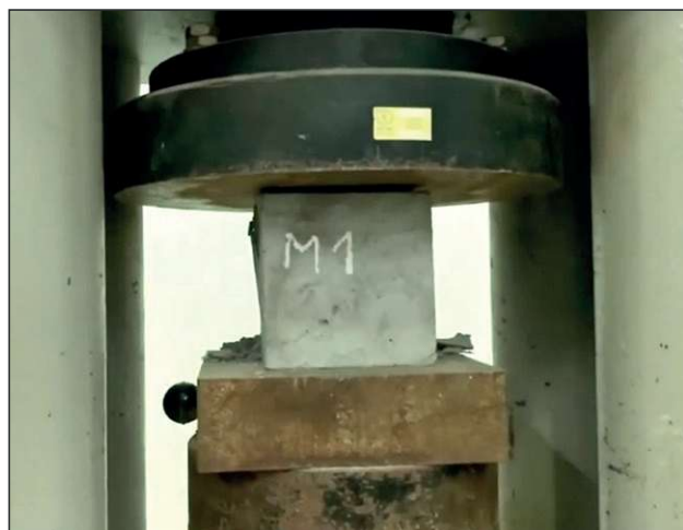
Fig. 10. Compression testing of concrete samples
