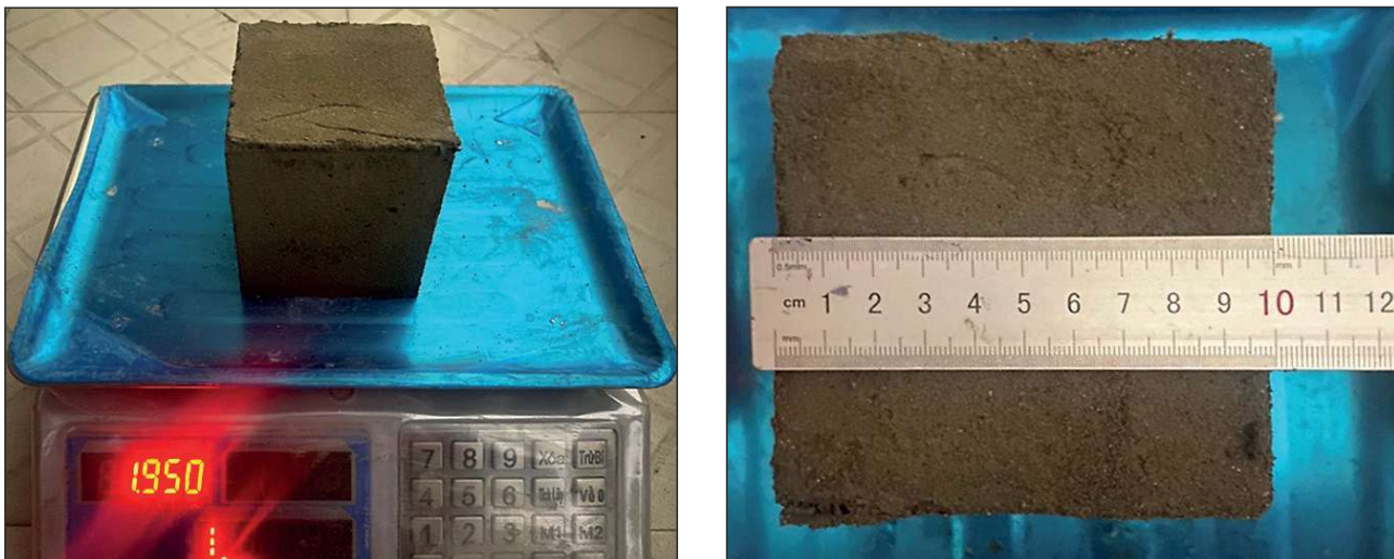
Fig. 12. Determination of the average density of developed concrete at the age of 28 days
