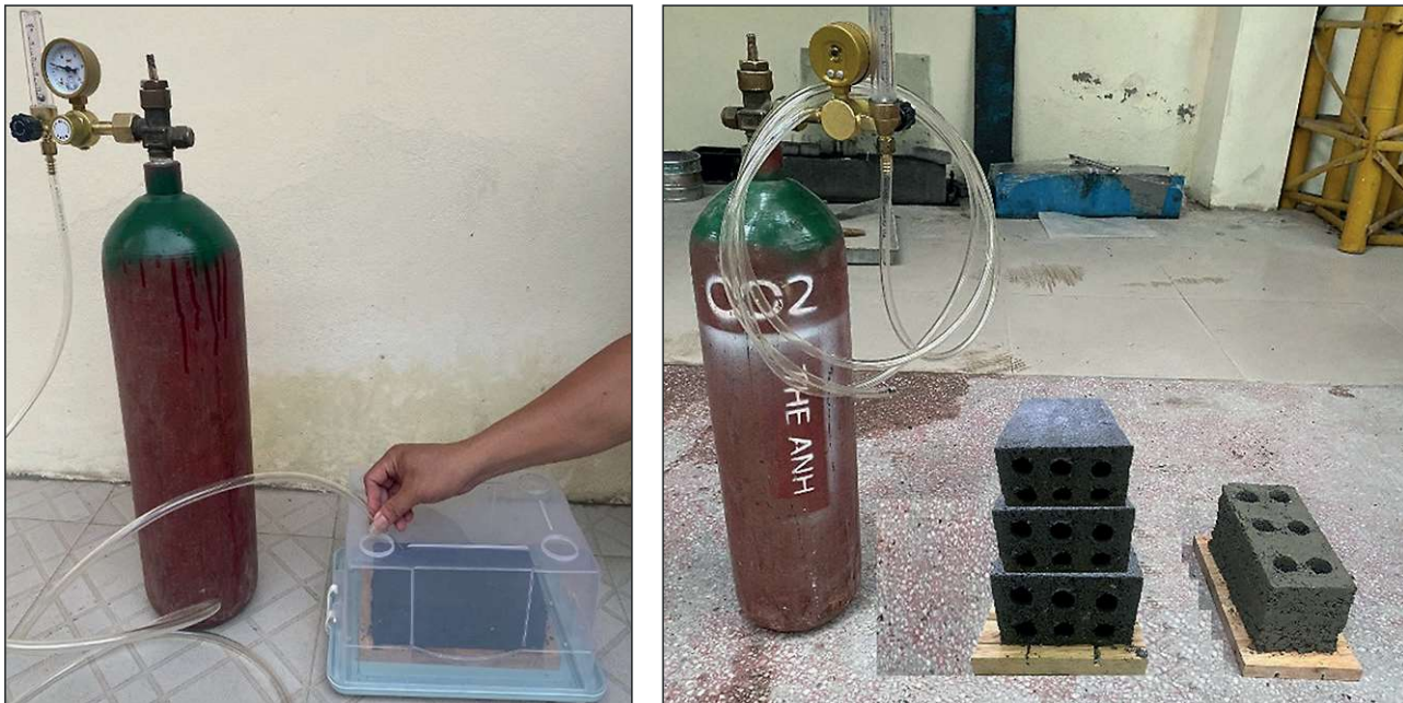
Fig. 11. Carbonation of samples of developed concrete during their hardening
