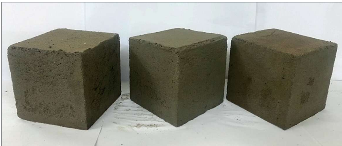
Fig. 9. Samples-cubes measuring 100×100×100 mm made of developed cement-free “green” concrete
