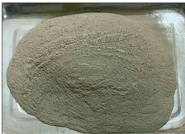
Fig. 6. Slurry waste from alumina production
