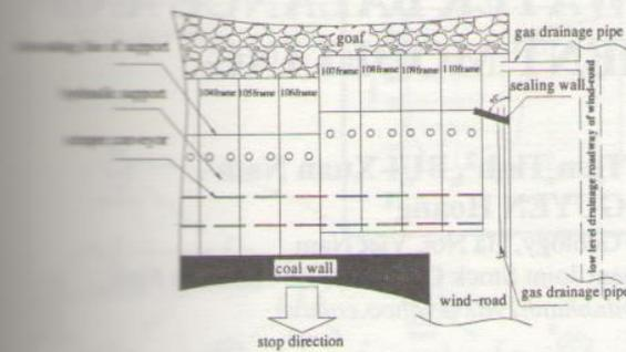
Fig.3. Schematic diagram of network drainage
