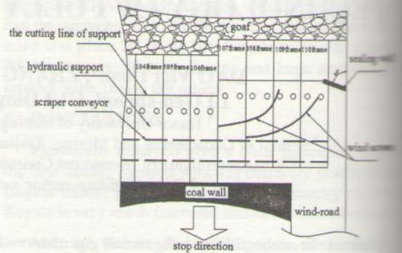
Fig. 2. Schematic diagram of wind screen
