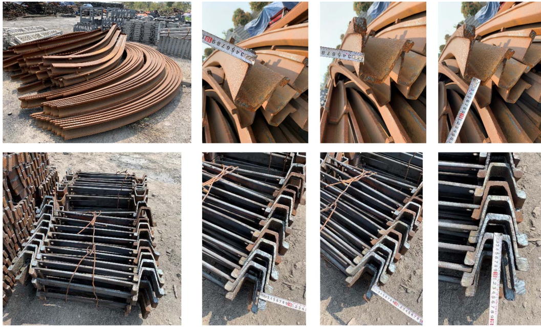
Fig. 12. U-Beams in Tunnels and the Measurement of Their Dimension Using a Tape
