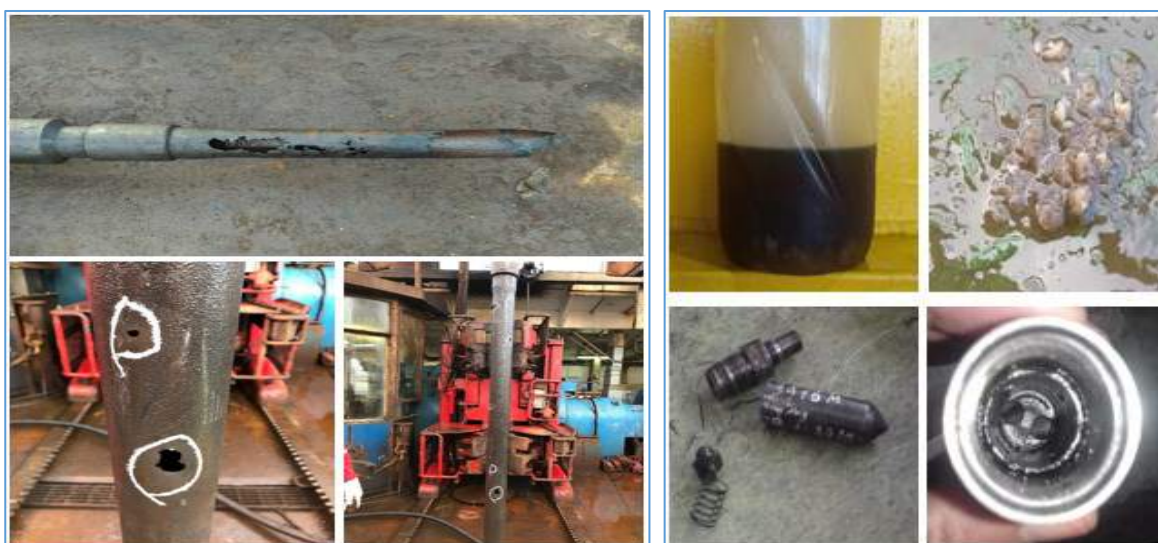
Fig 6. Results of salt treatment with acid and inhibition in wells 6X/ThTC-2 and 33P, 37P/ThTC-3).
