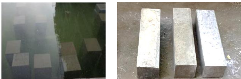
Fig. 6 – Specimen prepared for compressive and flexural tests
