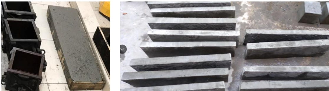
Fig 17 – Manufacturing concrete laggings in HUMG
