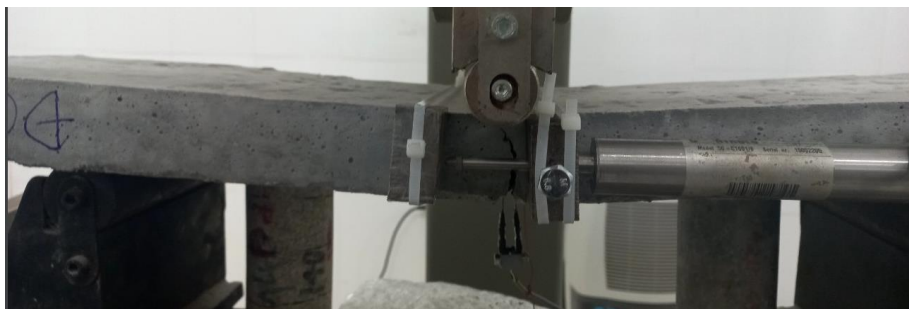
Fig 19 – The three-point load method for concrete lagging
