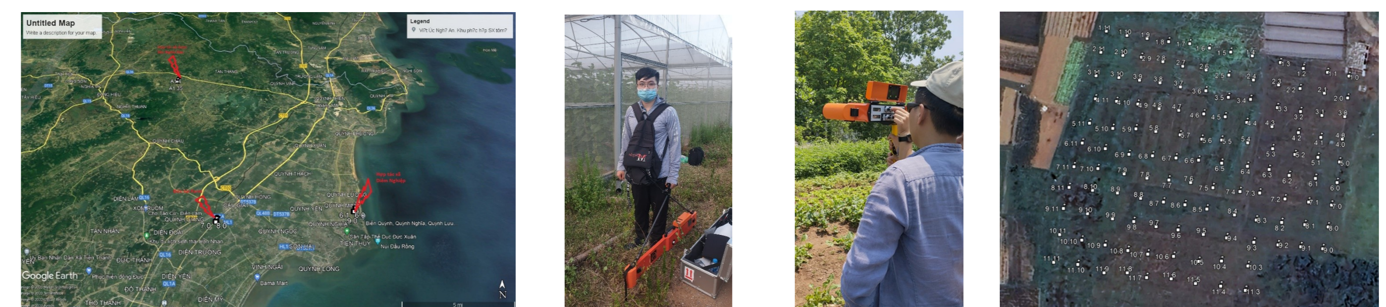
Figure 7: Field trips at Nghe An province: a) locations; b) EM38-MK2 instrument; c) equipment calibration; d) a map of measurement points at Diem Nghiep Farm
