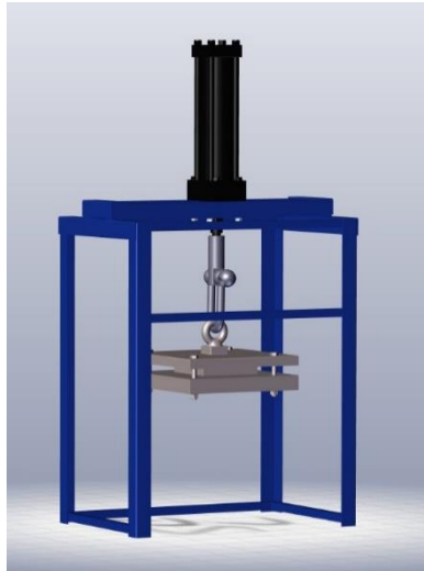
Figure 4 – A bottom up hydraulic cylinder plays as a displacement pump (source cylinder)
