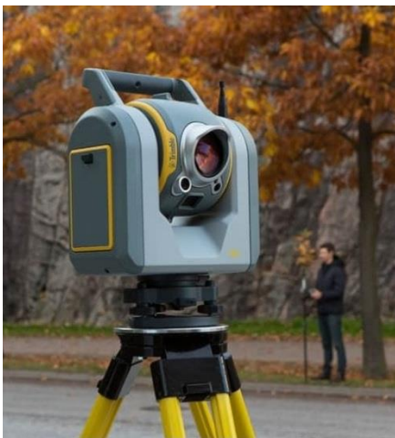
Quét 3D Scan Trimble SX10
