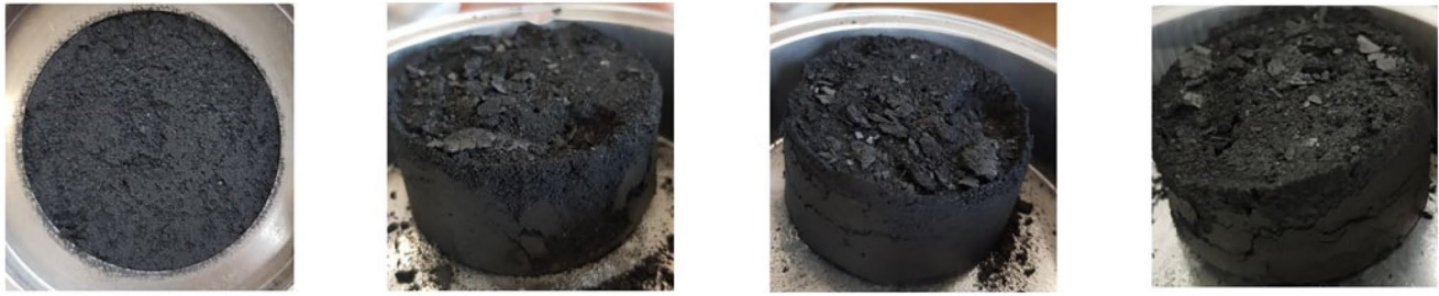
Figure 10. The specific case indicate the cracks that divide the filter cake into two sections horizontal.
