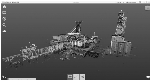
Fig. 9. TLS point clouds for mine shafts (shown in RECAP software)
