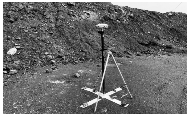
Fig. 7. Measurement of GCPs using the GNSS/T300 receiver
