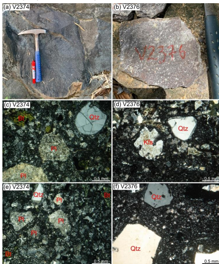
Fig. 2. Field images of rhyolite (sample V2374) and rhyolite porphyry (sample V2376) and microphotographs from their thin sections under a microscopy (magnification of 5x).
