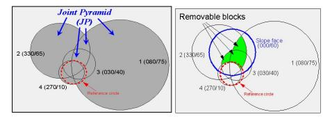
Figure 3. Identification of removable blocks on stereonet.
