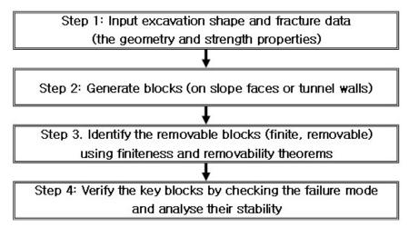
Figure 2. Steps of key block analyses.
