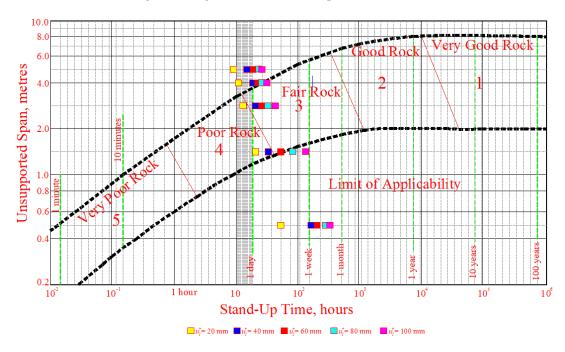
**Figure 11.** Relationship of unsupported tunnel span with stand-up time corresponding to various values of allowable displacement of tunnel.
