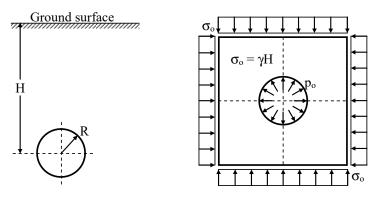
Figure 5. Mechanical model for tunnel excavation, adopted in this study.
