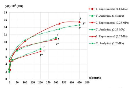
**Figure 4.** Relationship between rheological deformation and time, obtained by experimental and analytical approaches.
