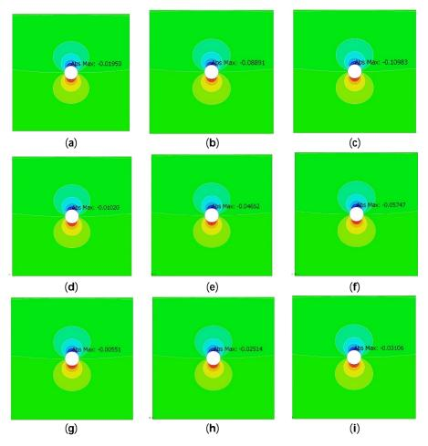
**Figure 9.** Vertical displacements of tunnel wall (**a**) at GSI 40, immediate reaction; (**b**) at GSI 40, after 200 h; (**c**) at GSI 40, after 500 h; (**d**) at GSI 50, immediate reaction; (**e**) at GSI 50, after 200 h; (**f**) at GSI 50, after 500 h; (**g**) at GSI 60, immediate reaction; (**h**) at GSI 60, after 200 h; and (**i**) at GSI 60, after 500 h. (heat map presents the displacement distribution).
