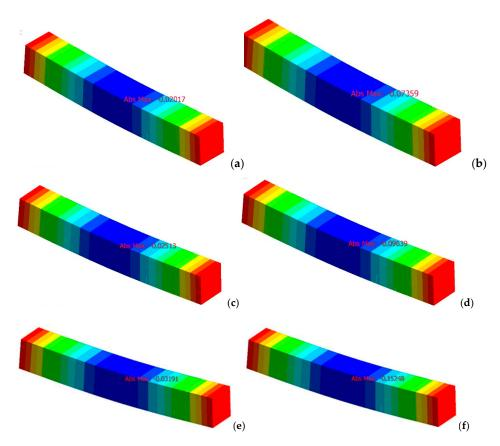
**Figure 7.** Beam deflection subjected to tensile stress of (a) 1.8 MP, immediate reaction; (b) 1.8 MPa, deflection after 200 h; (c) 2.25 MPa, immediate reaction; (d) 2.25 MPa, deflection after 300 h; (e) 2.7 MPa, immediate reaction; (f) 2.7 MPa, after 500 h. (where red color represent max. defection and blue represents min. deflection).
