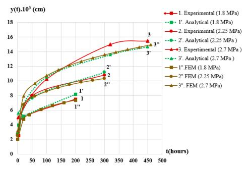
**Figure 6.** Comparison of results on rectangular beam deflection in time, subjected to different ranges of tensile stress, obtained via three investigation approaches (experimental, analytical and FEM).
