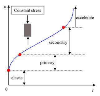
Figure 1. Creep response—a conceptual model of rheological curve.
