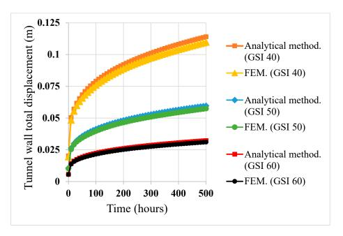
**Figure 8.** Total time-dependent displacement curves of tunnel walls gained using analytical and finite element methods according to various values of GSI (40, 50, 60).
