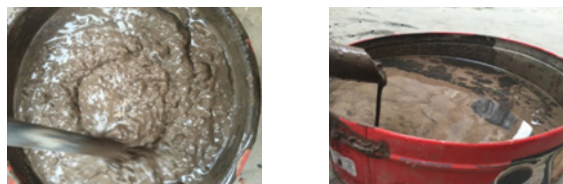
Fig. 7. Results of transport experiment in the pipeline: a. ratio of fly ash 18% &lt; b &lt; 30%, b. b &lt; 18% và b &gt; 30%
