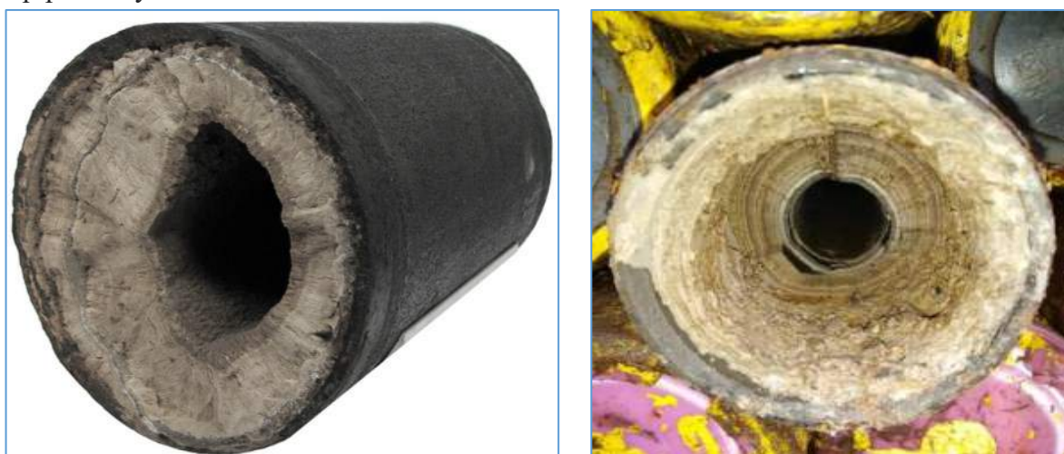
Fig 3. Salt deposits in the well and in a pipeline system.
