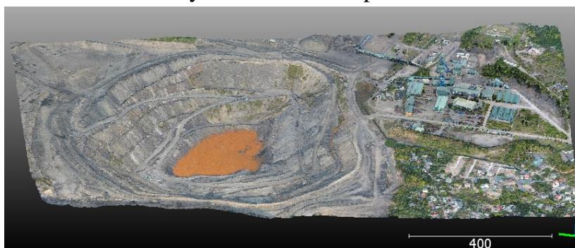
**Figure 8. 3D point cloud builded from UAV images**
