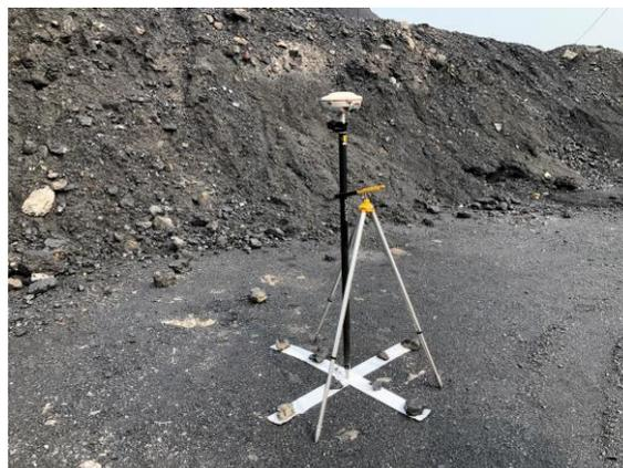
Figure 4. GCPs determination by GNSS/T300
