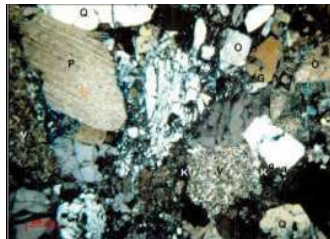
Sidewall core sample (at 3042m TVDs): arkose lithic sandstone with coarse grain, poor selectivity at well A1 (Q- quartz, P - Plagioclase)
