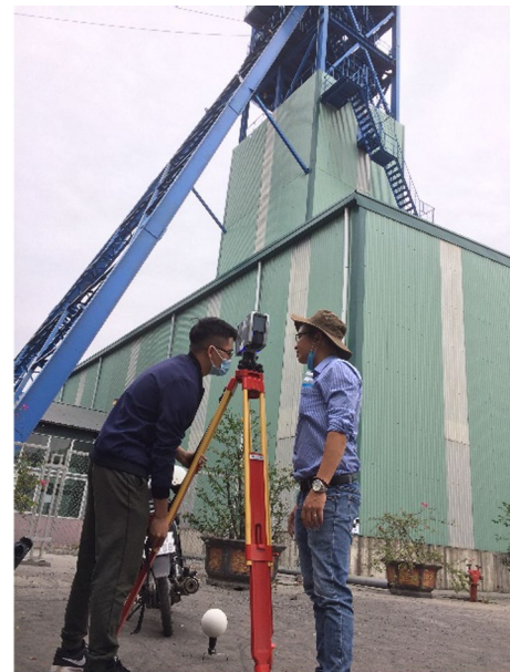
Fig. 8 Preparation of the FARO FOCUS3D X130 for scanning the study area
