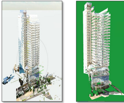
Fig. 7. Point clouds from TLS data
