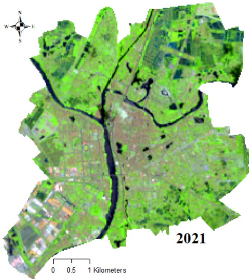
Figure 4. A Landsat composite image: vegetation (green), open water (dark blue); urban (brown).
