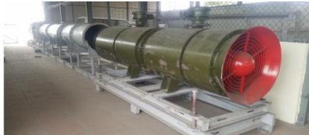
Fig. 3.1. Experimental apparatus for determination of duct resistance
