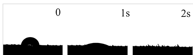
Figure 3. Water drop in delignified wood template
