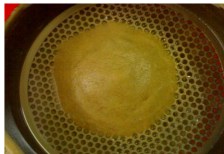
Figure 9d: The soil sample completely disintegrated after 15 seconds
