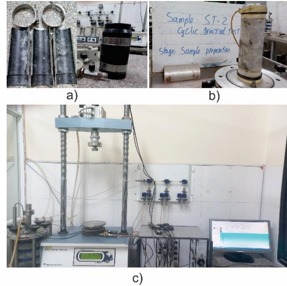
Fig. 3 a) Split mold for sample preparation; b) Sample after preparation; c) Triaxial apparatus
