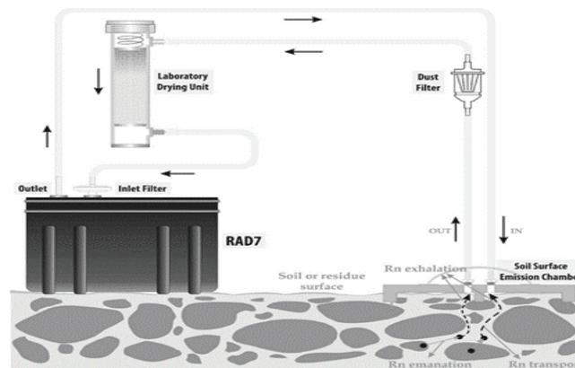
Fig. 2. A schematic layout of the installation used for radon distribution within soil depth.
