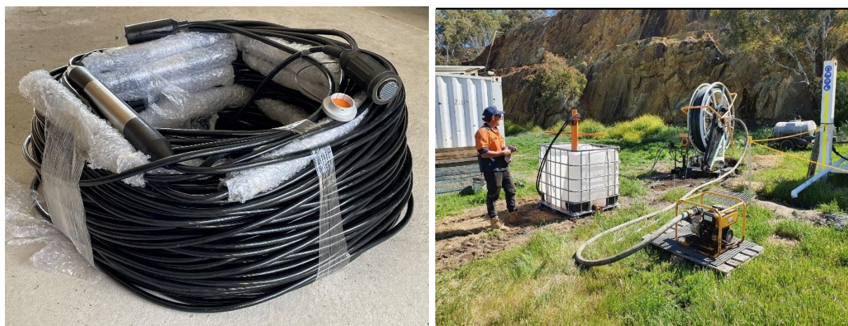
Figure 2. The 200m seismic string is pictured in the left panel and the (1-C and 3-C) sensor pods are 38mm diameter at 10m spacing. The strings are mounted on a tremie pipe and concrete-grout is pumped into the pipe until it flows out of the annulus of the hole at surface. This procedure is carried by the drilling crew in right panel and is compatible with current practice of sealing and completing holes in exploration.
