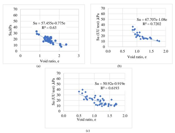
Figure 7 The relationship between undrained shear strength (Su)<sub>UU</sub> and void ratio (e) of soft soil at Thanh Hoa (a), Nghe An (b), Ha Tinh (c) in Vietnam's north central region
