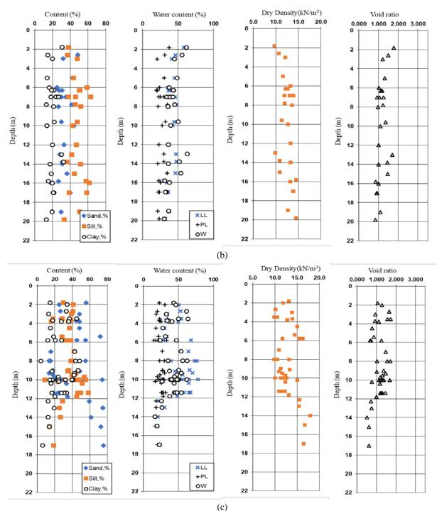
Figure 2 Some properties of soft soil at Thanh Hoa (a), Nghe An (b), Ha Tinh (c)
