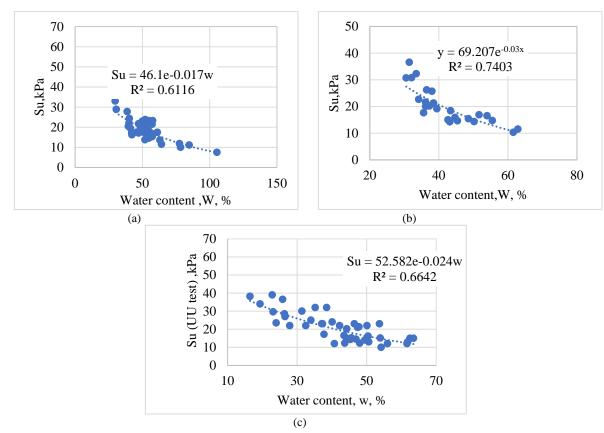
Figure 4 The relationship between undrained shear strength (Su)<sub>UU</sub> and water content (w) of soft soil at Thanh Hoa (a), Nghe An (b), Ha Tinh (c) in Vietnam's north central region
