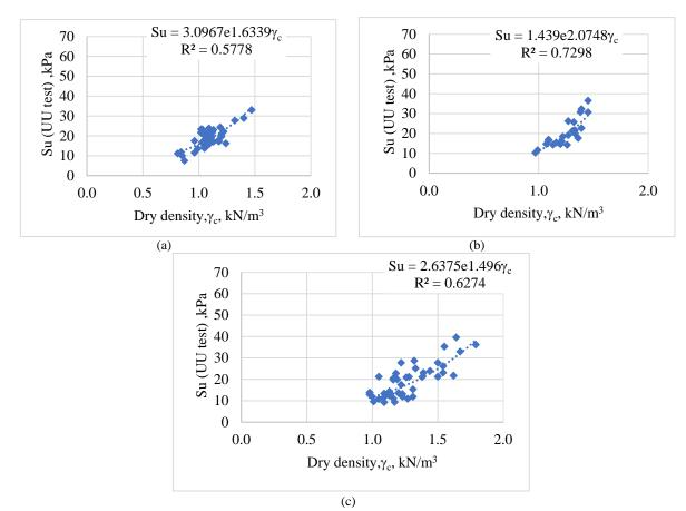
Figure 6 The relationship between undrained shear strength (Su)<sub>UU</sub> and dry density (γ<sub>c</sub>) of soft soil at Thanh Hoa (a), Nghe An (b), Ha Tinh (c) in Vietnam's North Central region
