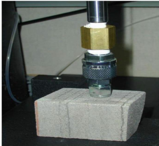
Figure 3. Probe-Permeameter During Permeability Measurements (Meyer, 2002).
