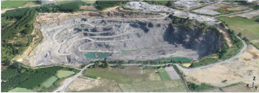
Fig. 2 3D texture model of the Thuong Tan 3 quarry, Vietnam in 2020 captured by DJI Phantom 4 Pro
