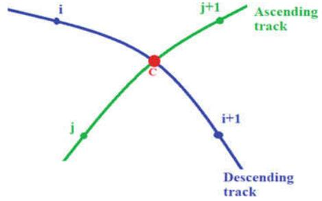
helps to find a suitable intersection. The position of the found intersection point is not an exact location, but an approximate location. After determining an approximate intersection point, four neighborhood points of the intersection  $i, i + 1, j,$  and  $j + 1$  from the ascending and descending tracks are determined (Fig. 2). From these 4 points, we will determine the position of the intersection point (C) more accurately.
