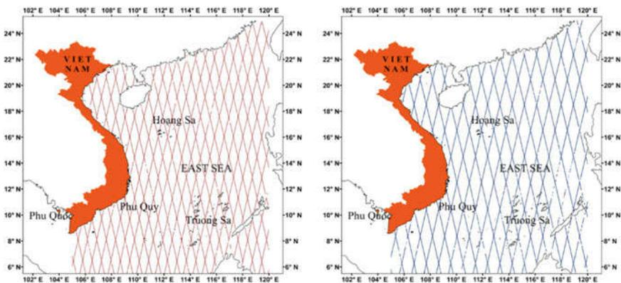
**Fig. 1** Track distribution of SARAL/AltiKa (left) and Sentinel-3A (right) satellites
