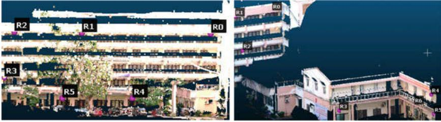
**Fig. 10** Scenario 5—CPs are evenly distributed on both PC1 (left) and PC2 (right)
