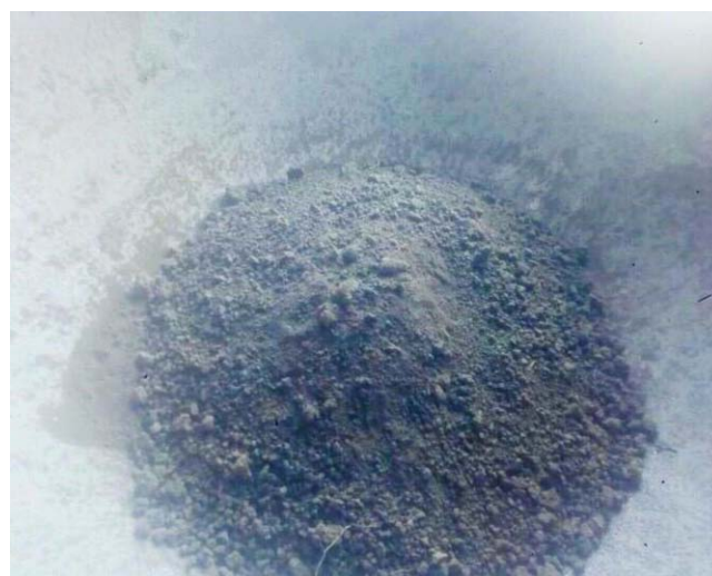
Figure 2. Processed MK sample at a calcination temperature of 650°C
