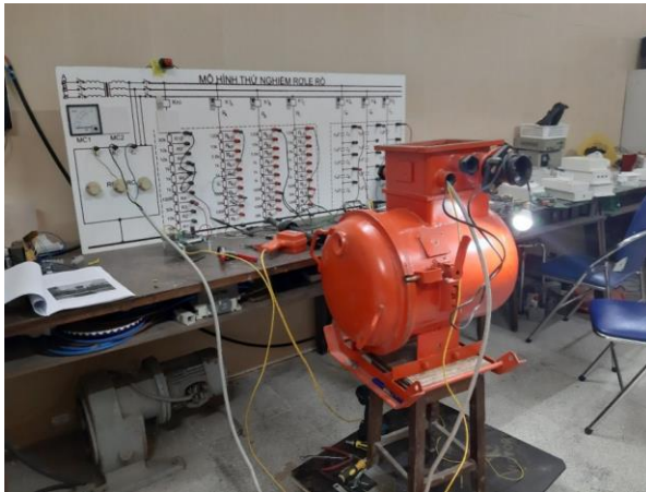
Figure 6. Experiment to determine the tripping resistance of earth leakage protective device
