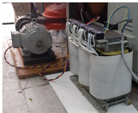
Figure 3. Devices for generating back e.m.f of the motor when the power is cut off
