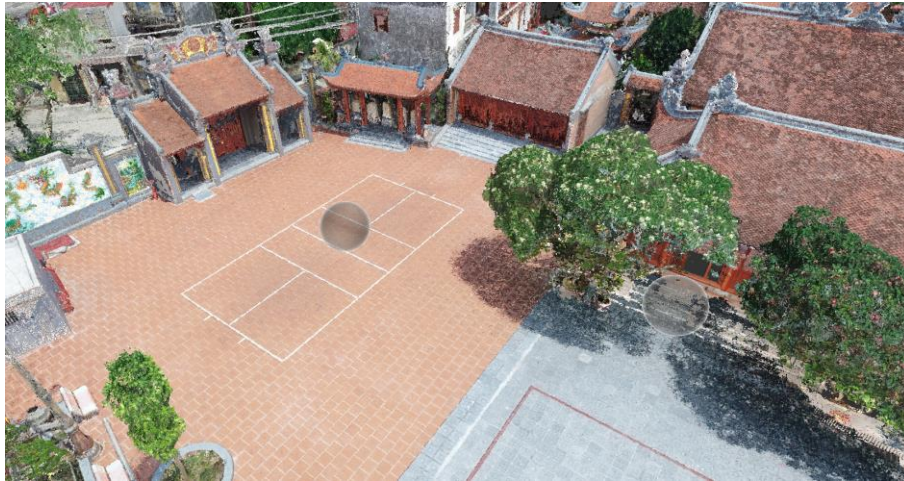
Figure 8. TLS and UAV point cloud data stitched together.
