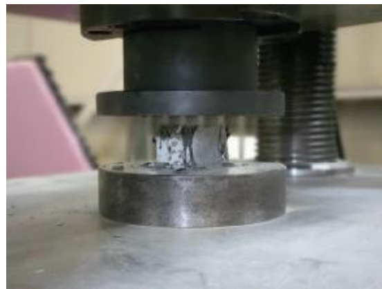
Figure 6. The failure of smart UHPC specimen under compression.
