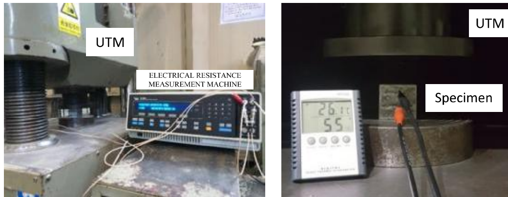
Figure 4. Test setup for measuring electrical resistance of specimens during compressive loading.
