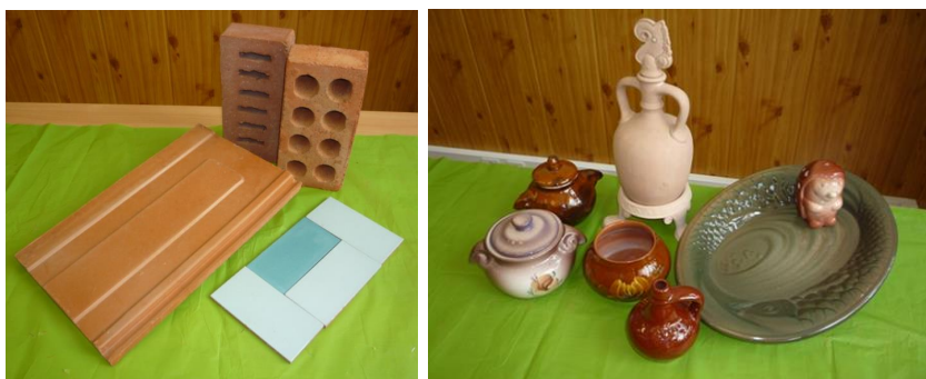
Fig. 1. Prototypes of ceramic products from technogenic raw materials
