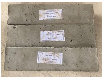
Figure 4. Flexural strength test samples.
