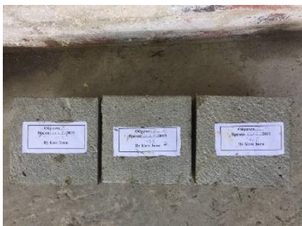
Figure 5. Compression test samples.
