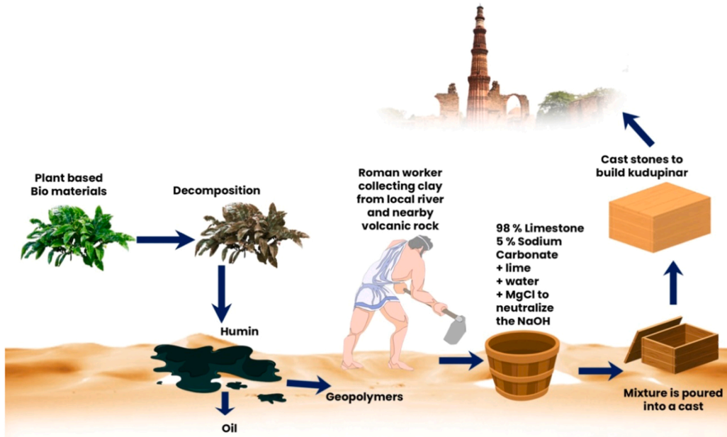
Fig.-5. Geopolymer used in kudupinar monument construction.
