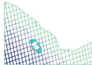
FIGURE 8. Axial force and moment in upporting structure of the tunnel
