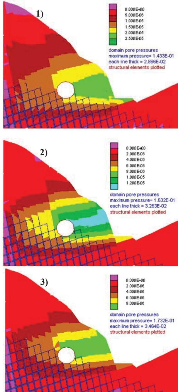
**FIGURE 7.** Dependent of horizontal Displacement and pore pressure on water level above the top of the tunnel: 1) 0m; 2) 2m and 3) 3m.
