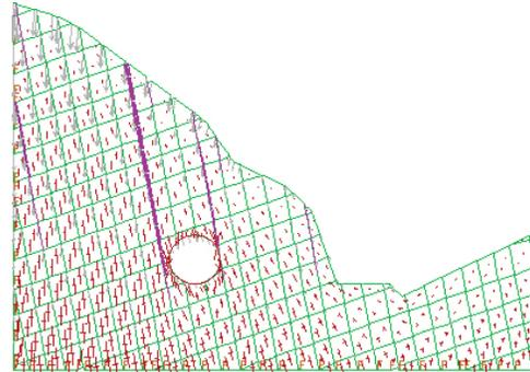
FIGURE 5. Displacement and stress in supported tunnel
