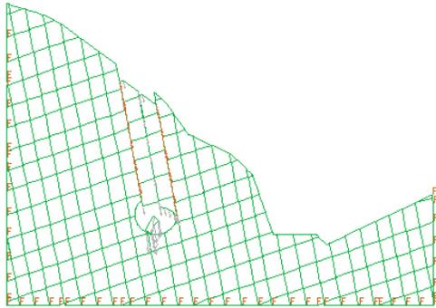
FIGURE 4. Rock Failure in unsupported tunnel
