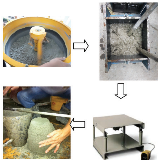
Figure 2. Procedure for preparing mixtures.
